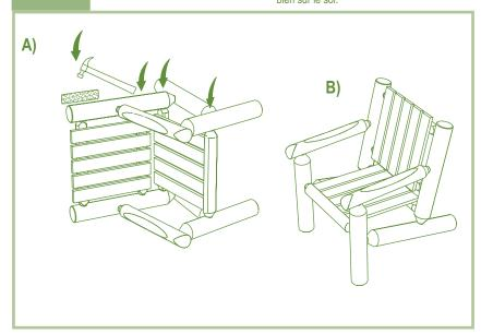
Screw the joints... Screw the joints at a Screwing is the same on the left perpendicular angle only. and right sides.
